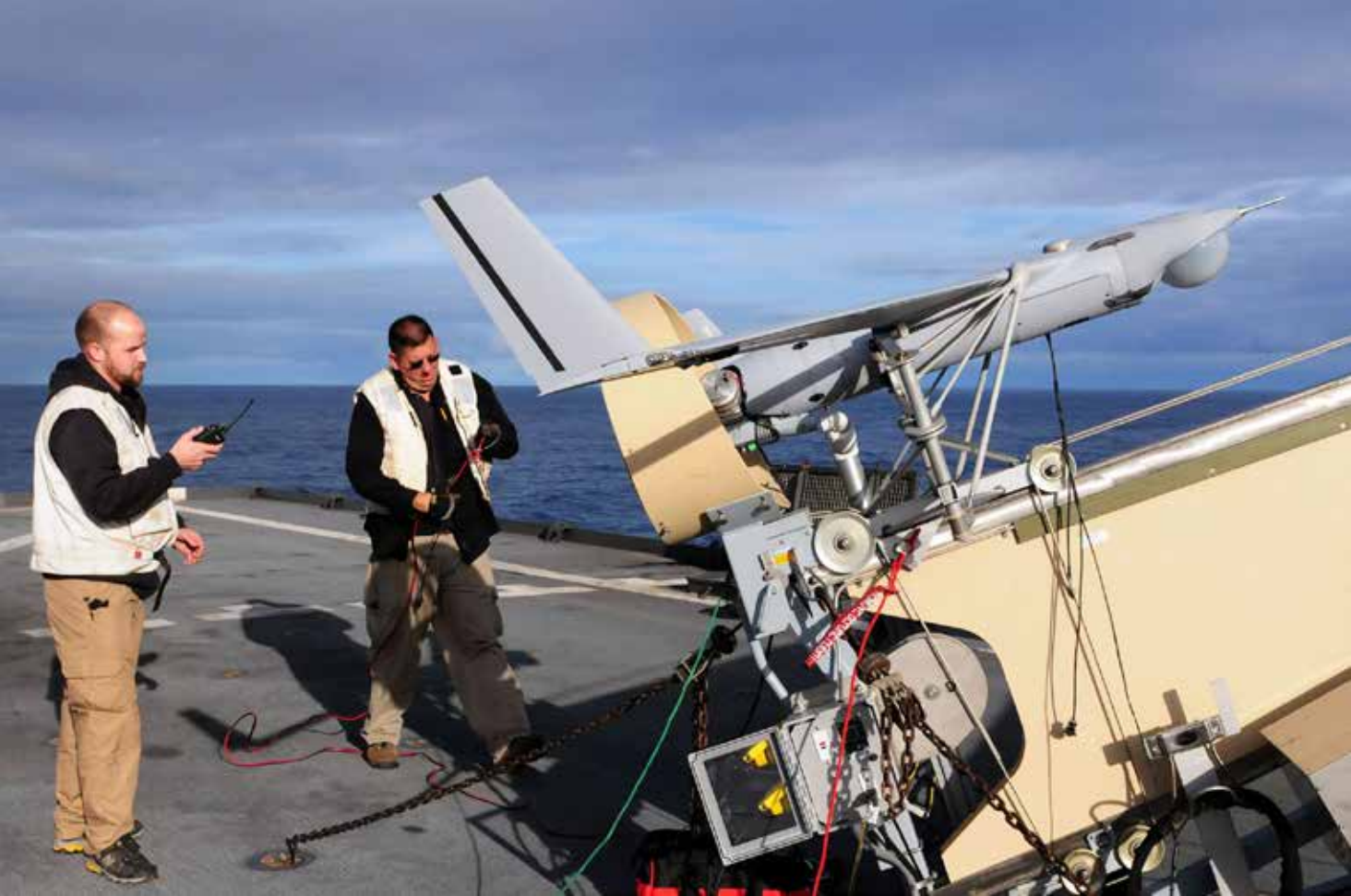
Guy McAllister from Insitu, left, and Jason Wolfram from Boeing Inc. perform preflight checks on a ScanEagle before launch aboard the amphibious dock landing ship USS Comstock.
