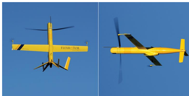
Flexrotor in rotorborne vertical flight (left) and wingborne horizontal flight (right). Credit: Aerovel
