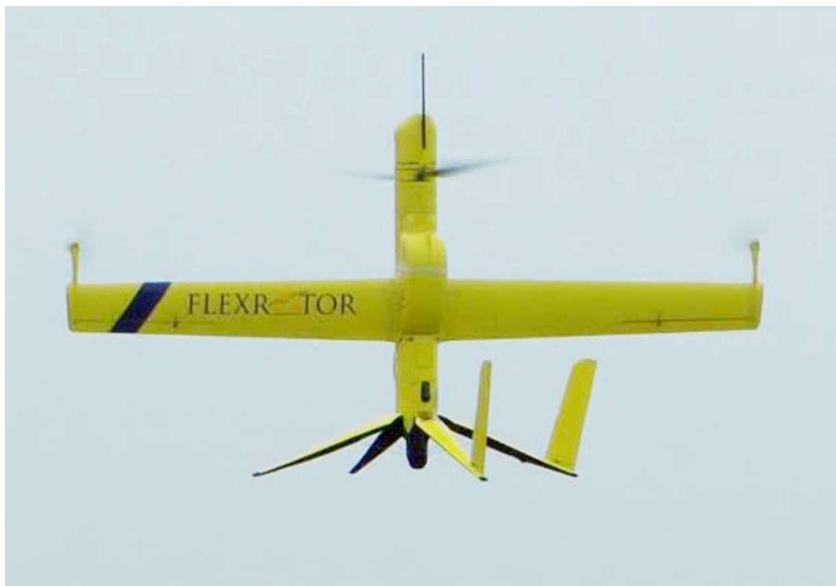
Flexrotor prepares to fold its landing gear after taking off on a flight that lasted more than 32 hr. Credit: Aerovel
