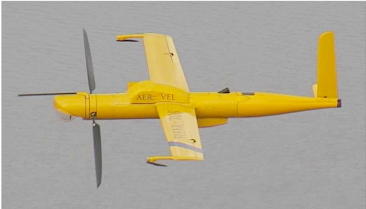
Flexrotor transitions to fuel-efficient wingborne flight, with the proprotor providing thrust. Credit: AeroVel
