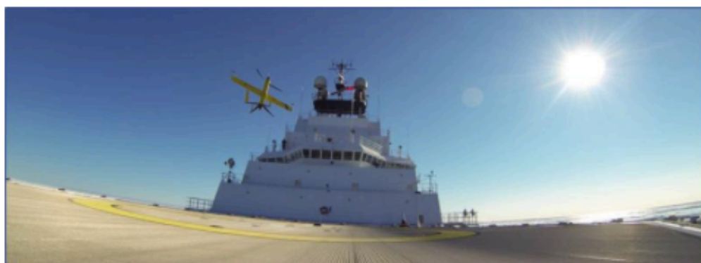
The VTOL aircraft's two-blade rotor becomes a propeller in wingborne flight, extending endurance. Credit: Aerovel
